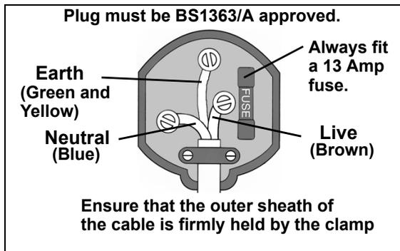
connected to the terminal which is marked E or
